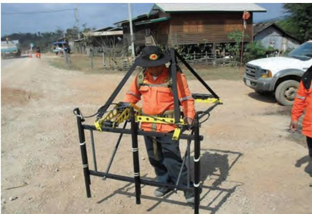
Foerster 4032 Triple Probe Setup for road clearance
